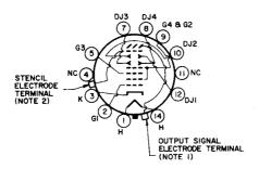
Pin No.1: Heater Pin No.2: Grid No.1 Pin No.3: Cathode Pin No.4: No connection Pin No.5: Grid No.3
