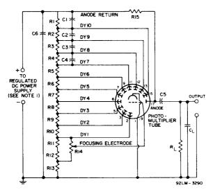
C<sub>1</sub>: 0.05  $\mu$ F, 500 volts C<sub>2</sub>: 0.02  $\mu$ F, 500 volts C<sub>3</sub>: 0.01  $\mu$ F, 500 volts C<sub>4</sub>: 0.005  $\mu$ F, 500 volts C<sub>5</sub> and C<sub>6</sub>: 0.005  $\mu$ F, 3000 volts
