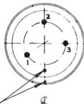
INDEX MARKS WILL BE DIAMETRICALLY OPPOSITE YELLOW LEAD AND WILL NOT DEVIATE FROM A COMMON  $\phi$  BY MORE THAN 15° IN EITHER DIRECTION
