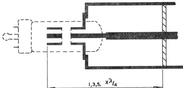
(B) VALVE WITH SHORT CIRCUIT COAXIAL LINE: COAXIAL CAVITY.
