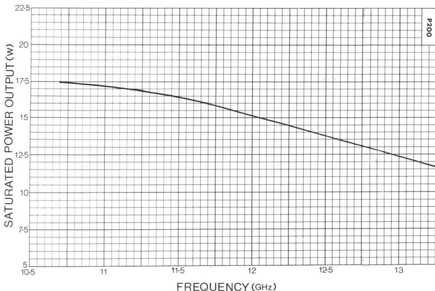
Fig. 2. Typical Synch. Gain at Working Output versus Frequency
