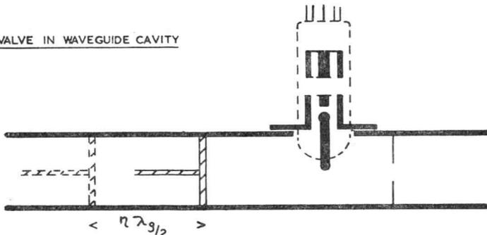
Fig. 3.—Basic Resonator and Cavity Structure
