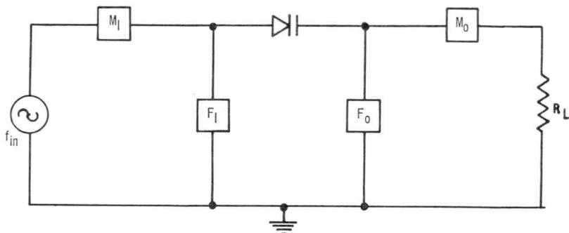
$F_I$  = Filter circuit, resonant at input frequency.
