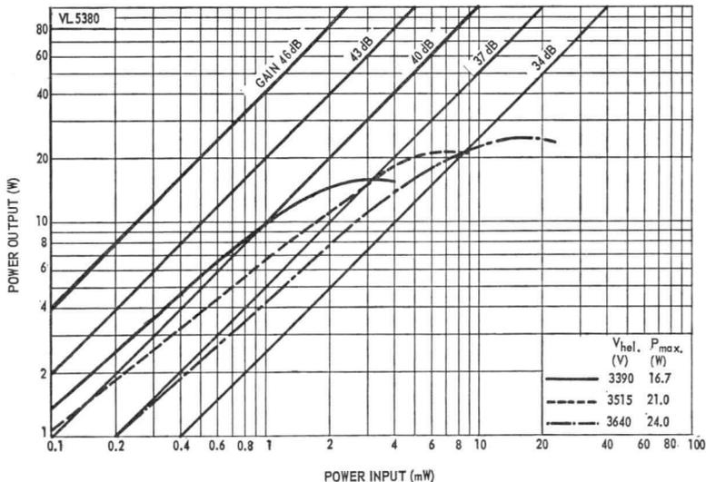
Fig. 4.—Typical Power Output versus Power Input at 7.8 GHz
