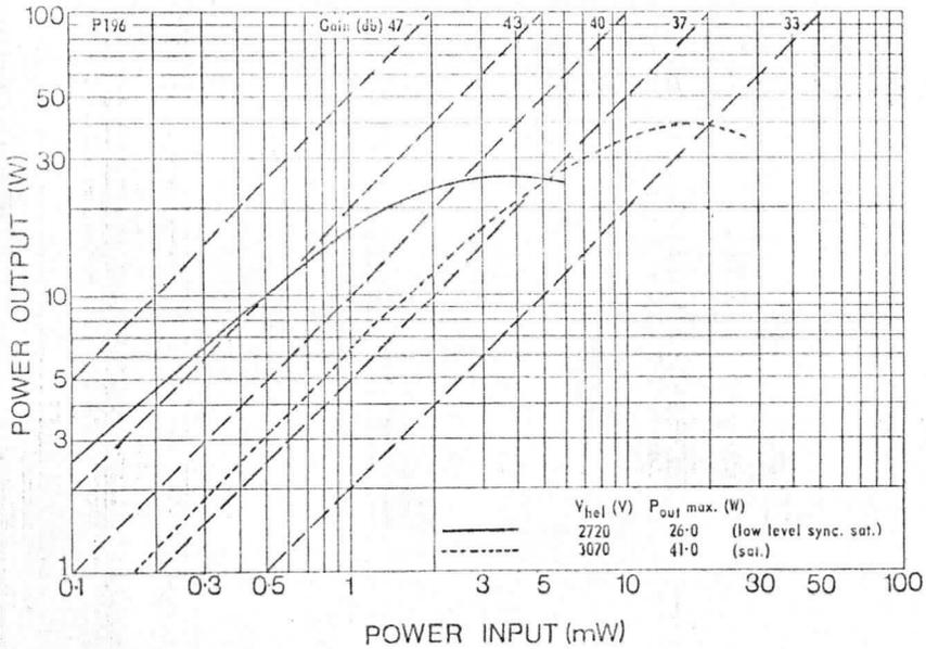
Fig. 5. W7/6GA Typical Power Output versus Power Input at 4.2GHz
