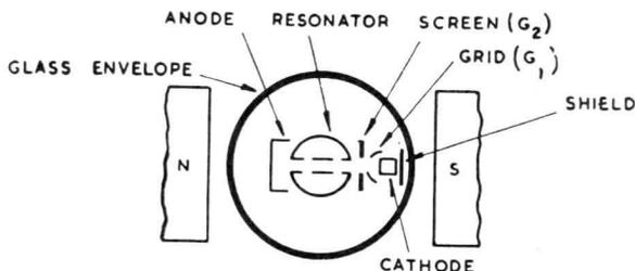
Fig. 1.—Cross section of valve assembly
