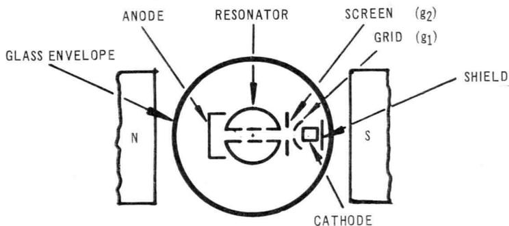
Fig. 7.—Typical Tuning Cavity
