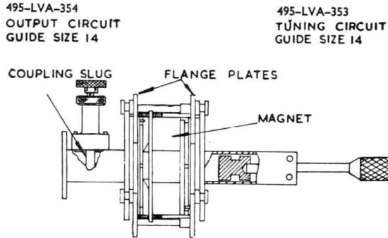
Fig. 5.—Cross-section of Cavities
