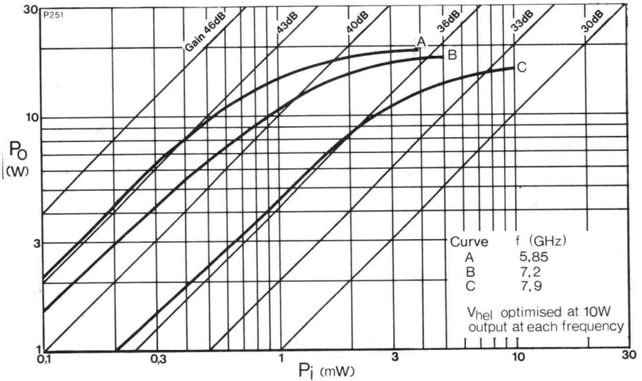
Fig. 3. Typical Output Power versus Input Power - W5/4GC
