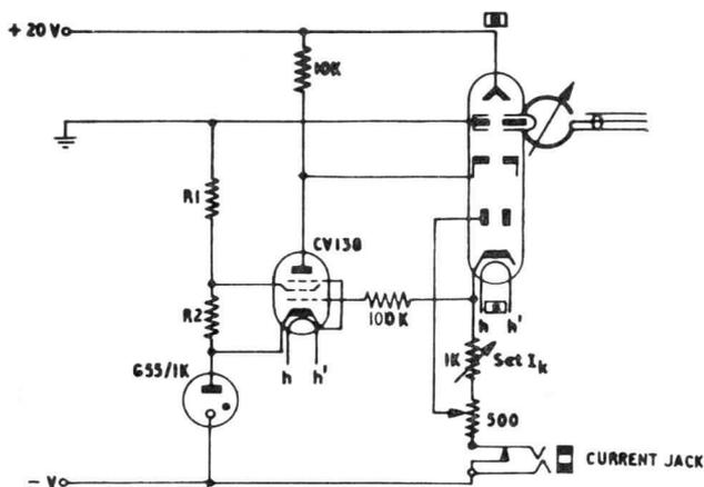
Fig. 2.—Circuit for stabilisation of V.M. oscillator tube current
