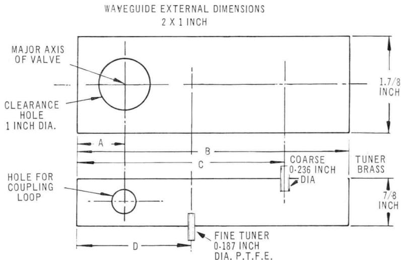
TRAVEL OF SLUGS JUST LESS THAN 7/8 INCH TO PREVENT CONTACT WITH OPPOSITE WAVEGUIDE WALL.
