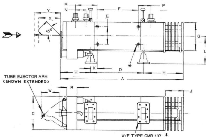
DIM-X (WITHDRAWAL DISTANCE OF TUBE WITH LATERAL MOVEMENT OF BASE) 10" MIN.
