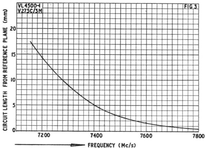
Fig. 4.—Typical Electronic Tuning Characteristic.
