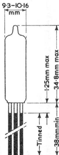
The bulb dimensions of this tube are in accordance with BS448, Section B8D.
