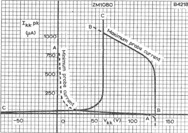
PEAK PROBE CURRENTS TO INDIVIDUAL CATHODES. PULSED ANODE
