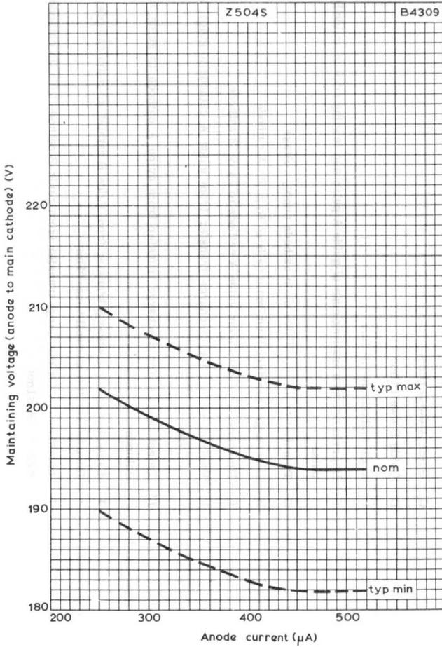
ANODE TO MAIN CATHODE MAINTAINING VOLTAGE PLOTTED
