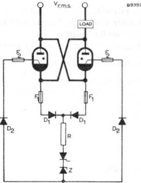
Fig. 2: Anode excitation (Common thyristor)
