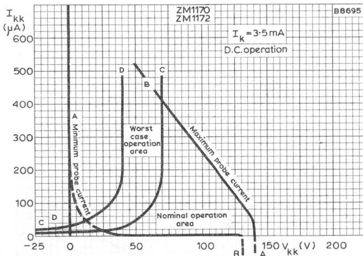
PROBE CURRENT TO INDIVIDUAL NON-CONDUCTING CATHODES
