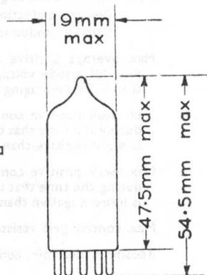
The bulb and base dimensions of this valve are in accordance with BS 448, Section B7G
