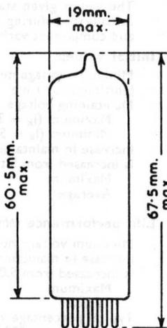
The bulb and base dimensions of this tube are in accordance with BS448, Section B7G
