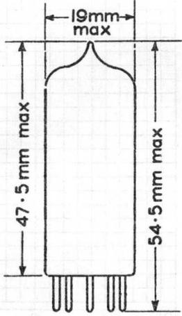
The bulb and base dimensions of this valve are in accordance with BS448, Section B7G
