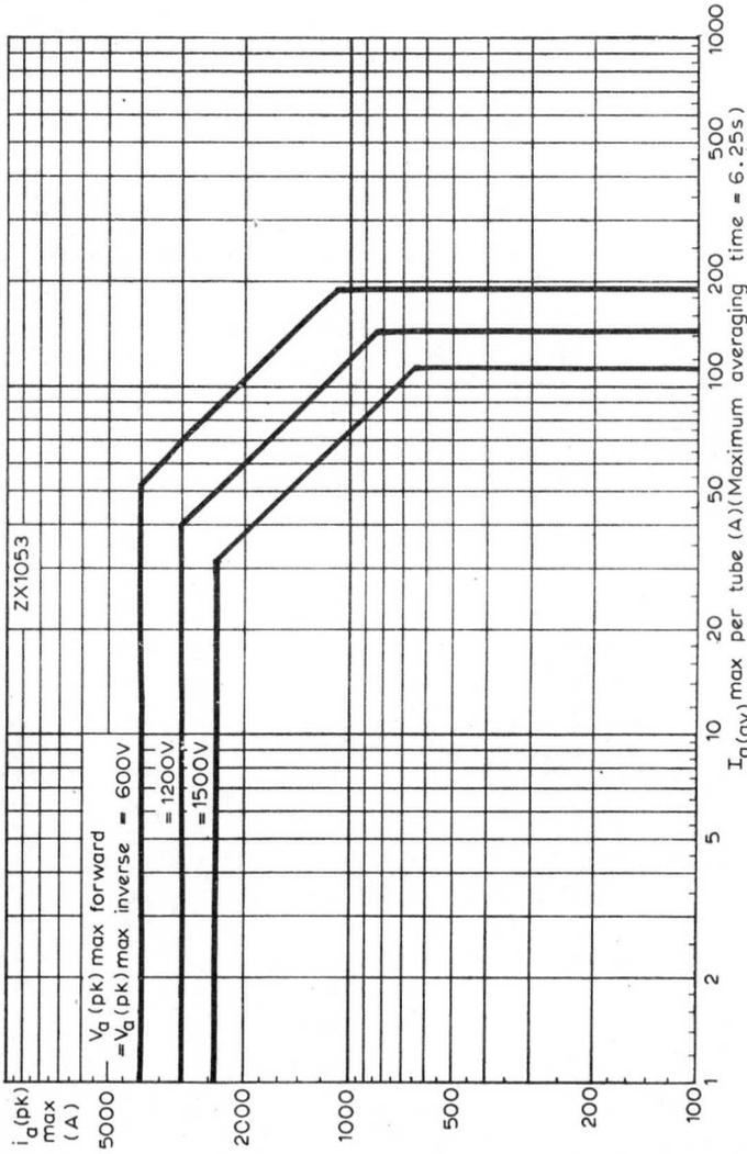
MAXIMUM PEAK ANODE CURRENT PLOTTED AGAINST AVERAGE ANODE CURRENT. INTERMITTENT RECTIFIER SERVICE
