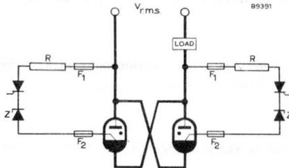
The "Min. peak ignitor voltage for ignition", must not be interpreted as the instantaneous value of mains voltage at the instant of ignition, but as the voltage measured between the ignitor lead-in and cathode. The values of the resistors in the ignition circuit and the level of supply voltage should be chosen so that the prescribed value of voltage is applied to the ignitor.
