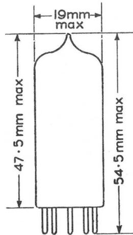
The bulb and base dimensions of this tube are in accordance with BS448, Section B7G.
