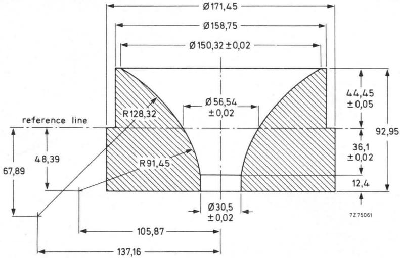
Fig. 4 Reference line gauge for 90° deflection angle.
