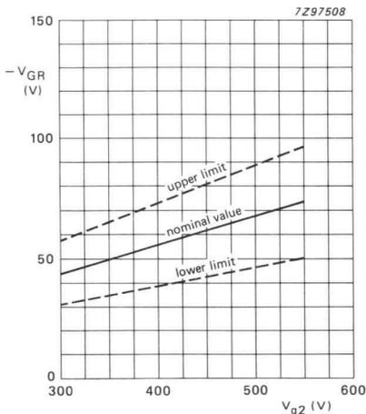
Limits of grid 1 cut-off voltage as a function of grid 2 voltage.
