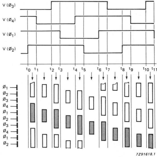
Fig. 2 Charge transport in the vertical direction.
