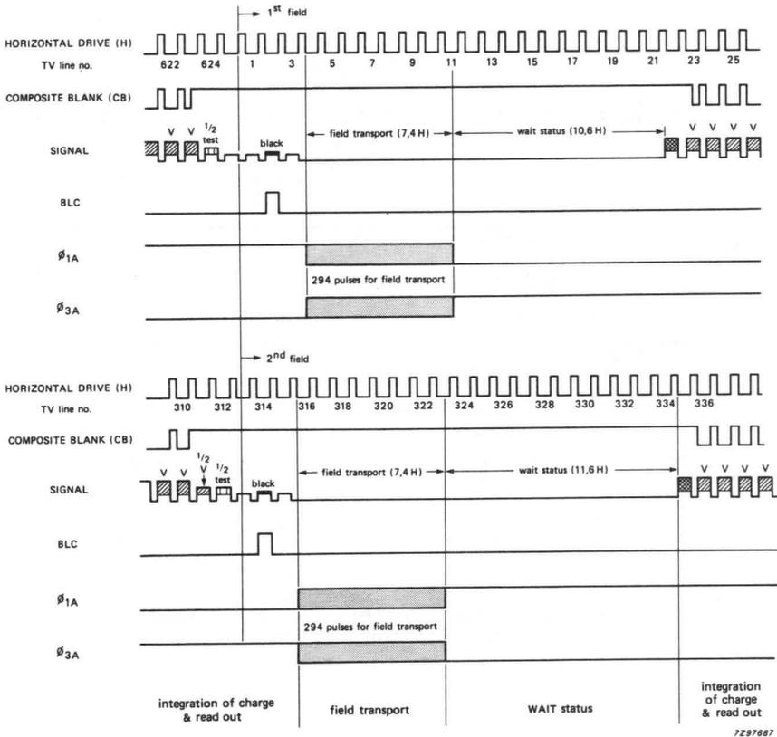
Fig. 8 Drive-pulse sequence and line numbering for field transport.
