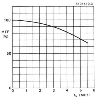
Fig. 14 Theoretical horizontal modulation transfer function; MTF as a function of the video signal frequency: three outputs correctly multiplexed.
