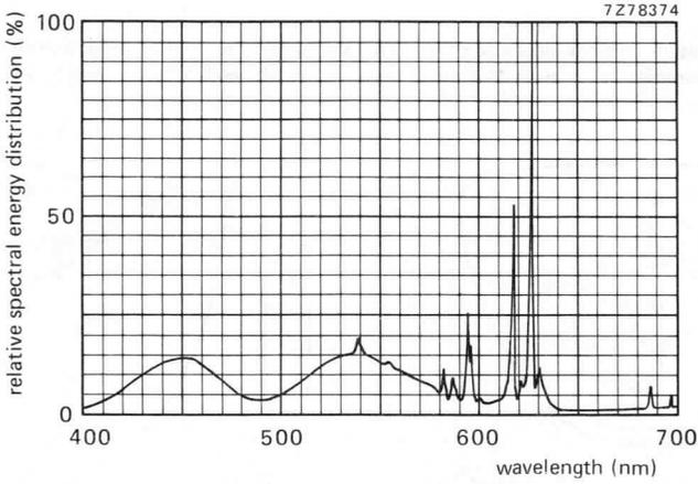
Fig. 17 Simultaneous excitation of red, green and blue phosphor, measured in a tube, to produce white of  $x = 0,281$ ,  $y = 0,311$ . Exact shape of the peaks depends on the resolution of the measuring apparatus.
