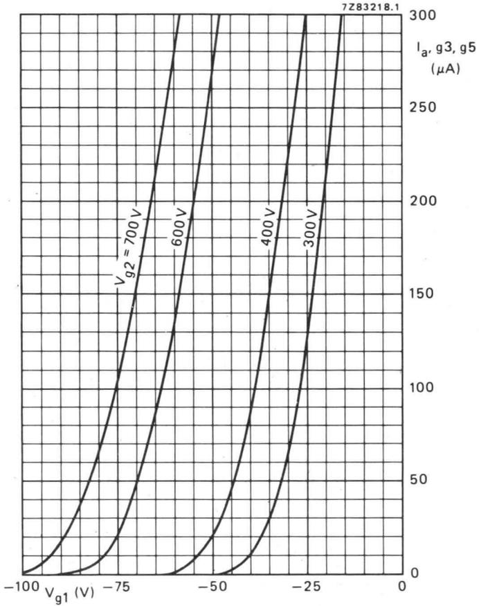
Anode current as a function of grid 1 voltage.
