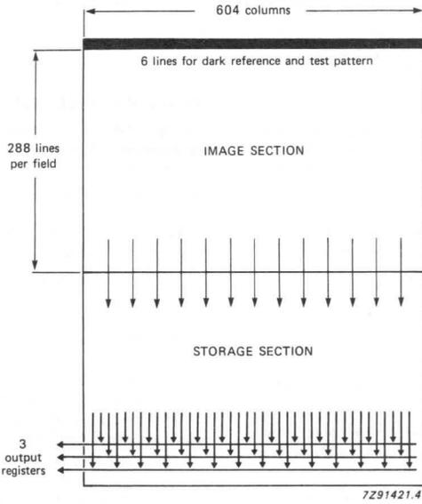
Fig. 1 Sensor layout and charge transport direction.
