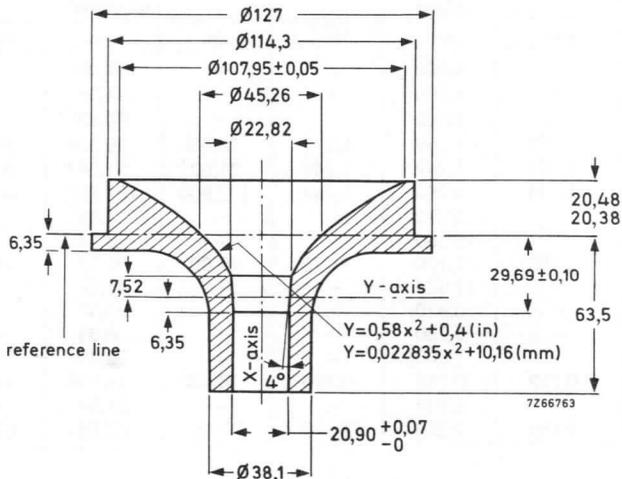
Fig. 3 Reference line gauge for 110° deflection angle.
