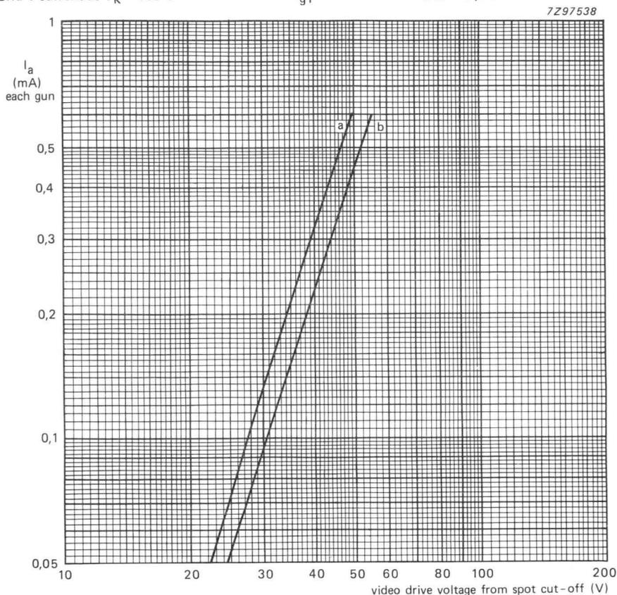
Fig. 14 Typical cathode drive characteristics at spot cut-off voltages of 80 V (curve a) and 105 V (curve b).
