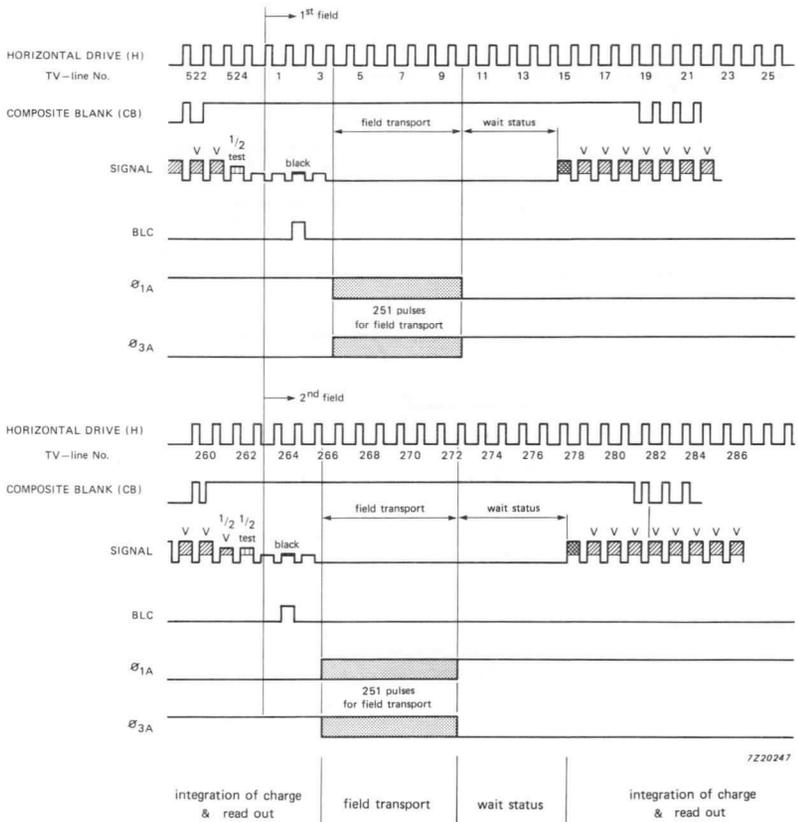
Fig. 8 Drive-pulse sequence and line numbering for field transport.
