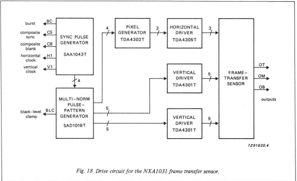
Fig. 18 Drive circuit for the NXA1031 frame transfer sensor.
