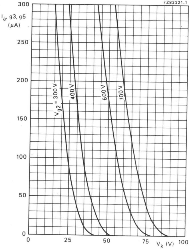
Anode current as a function of cathode voltage.
