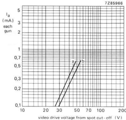
Fig. 13 Typical cathode drive characteristics at spot cut-off voltages of 85 V (curve a) and 105 V (curve b).
