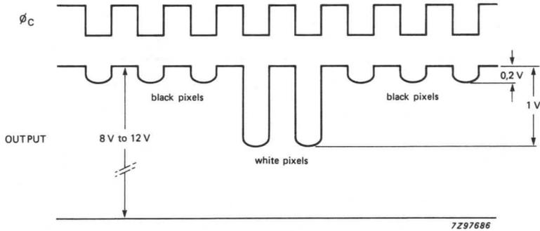
*Fig. 16 Typical signal at the sensor output.*
