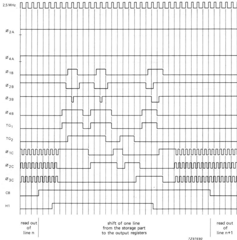
Fig. 12 Read-out of the output registers and sorting of the signal into output registers.
