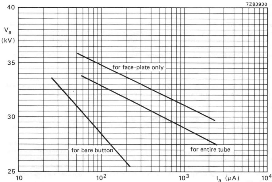
Fig. 15 0,5 mR/h isoexposure-rate limit curve.
