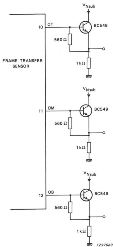
Fig. 5 Output buffer for measurements.
