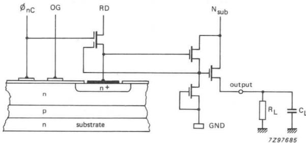
Fig. 15 Circuit diagram for one output channel.
