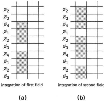
Fig. 3 Interlacing of the sensor.
