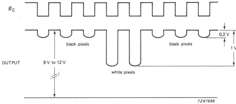
*Fig. 15 Typical signal at the sensor output.*
