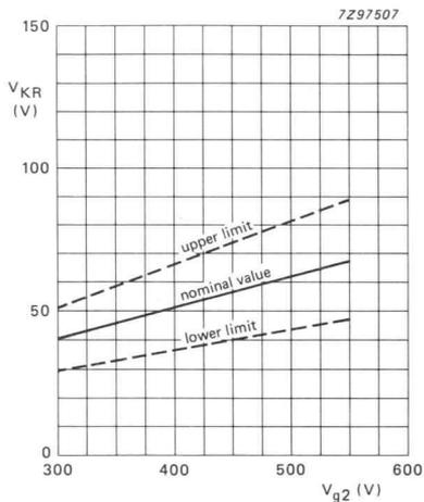
Limits of cathode cut-off voltage as a function of grid 2 voltage.
