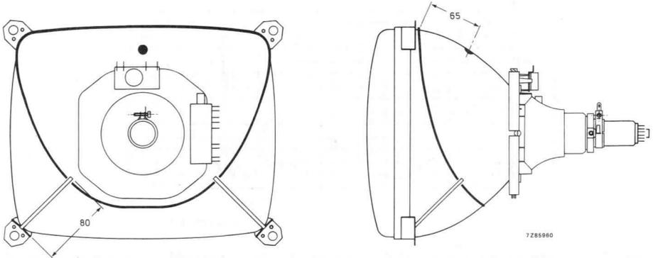
Fig. 18 Position of degaussing coil on the display tube; dimensions are given in mm.
