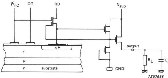
Fig. 14 Circuit diagram for one output channel.
