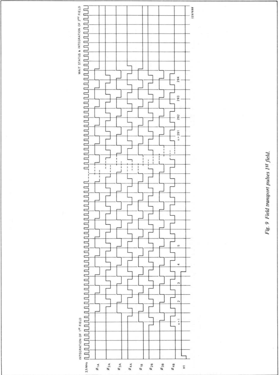
Fig. 9 Field transport pulses 1st field.
