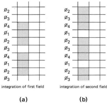
Fig. 3 Interlacing of the sensor.
