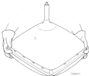
Fig. 3 Lifting picture tube from face-down position.
