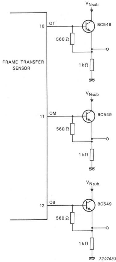
Fig. 5 Output buffer for measurements.
