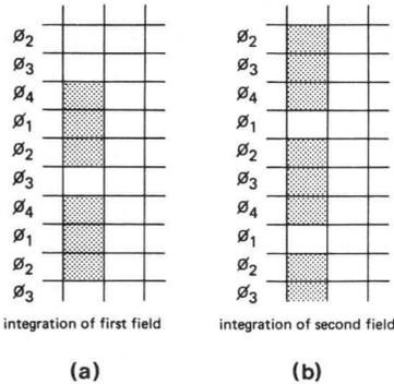
Fig. 3 Interlacing of the sensor.
