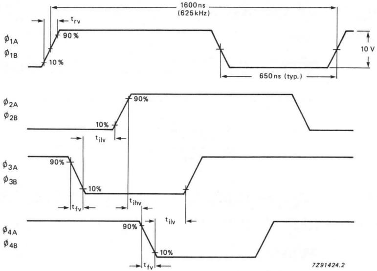
Fig. 7 Vertical transport timing waveforms for the sensor electrodes ( $\phi_{nA}$ ,  $\phi_{nB}$ ); times measured at the 10% and 90% points of the amplitude.
