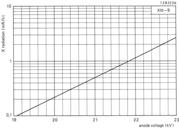
X-radiation limit curve according to JEDEC94, at a constant anode current of 250  $\mu$ A, measured according to TEPAC103A.
