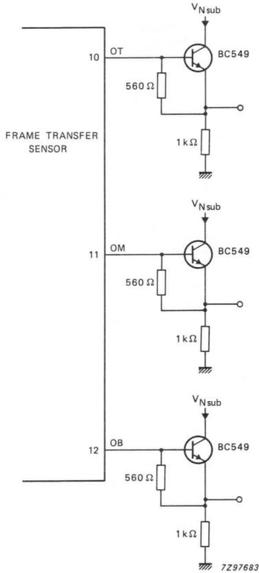
Fig. 5 Output buffer for measurements.
