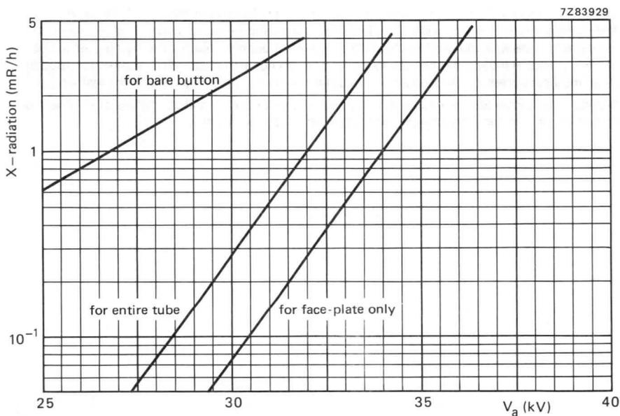
Fig. 16 X-radiation limit curve at a constant anode current of 300  $\mu A$ .
