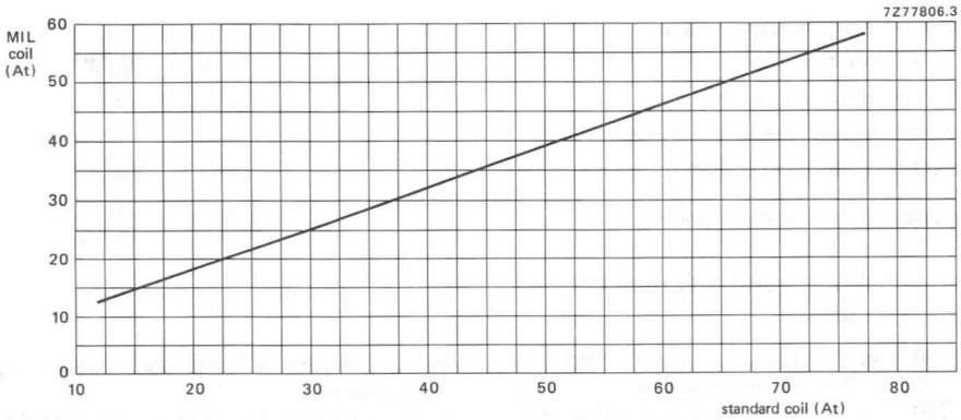
Fig. 2 Correlation at At operate in standard coil and MIL coil.
