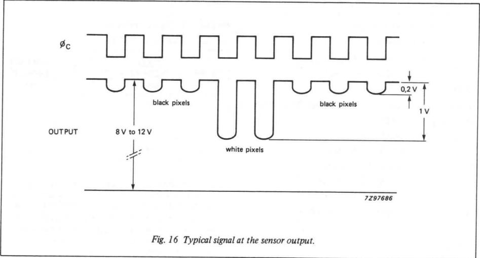
*Fig. 16 Typical signal at the sensor output.*
