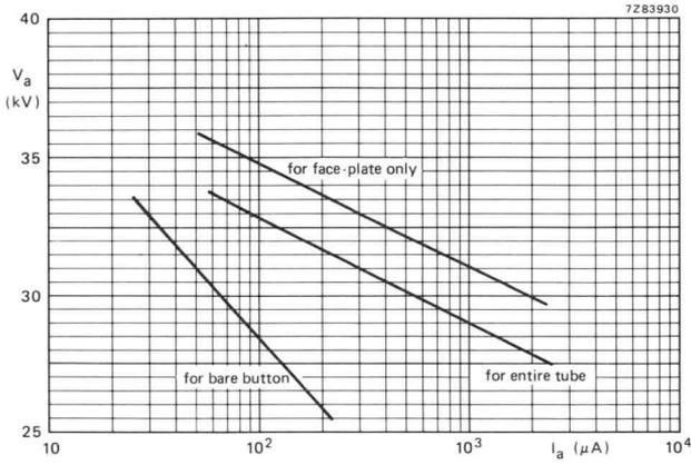
Fig. 16 0,5 mR/h isoexposure-rate limit curve.
