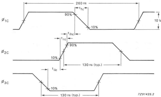
Fig. 6 Horizontal transport timing waveforms for the sensor electrodes ( $\phi_{nC}$ ); times measured at the 10% and 90% points of the amplitude.
