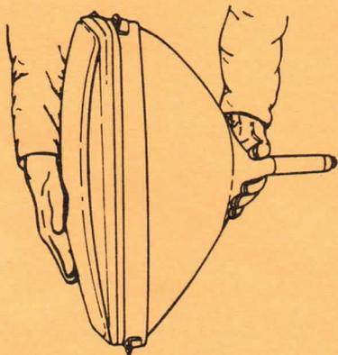
Fig.1 – Lifting tube from edge-down position.
