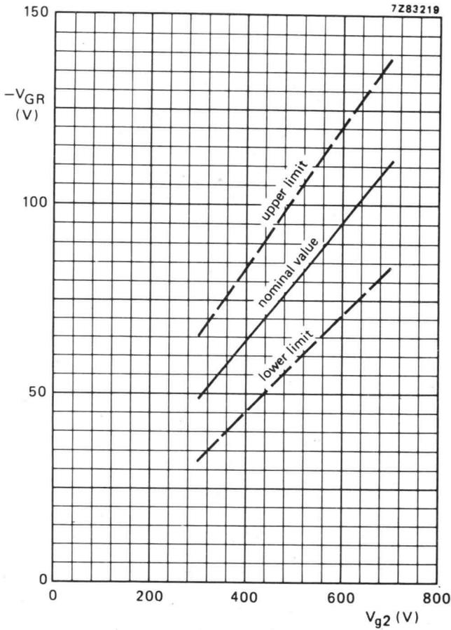
Limits of grid 1 cut-off voltage as a function of grid 2 voltage.
