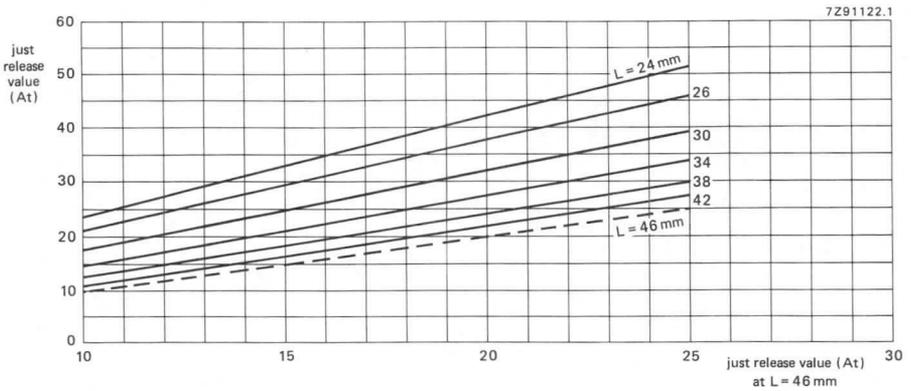
Fig. 5 Just release values at various overall length compared with standard length of 46 mm.
