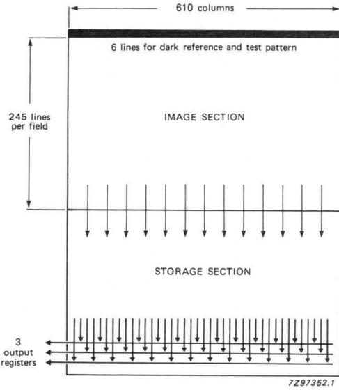
Fig. 1 Sensor layout and charge transport direction.
