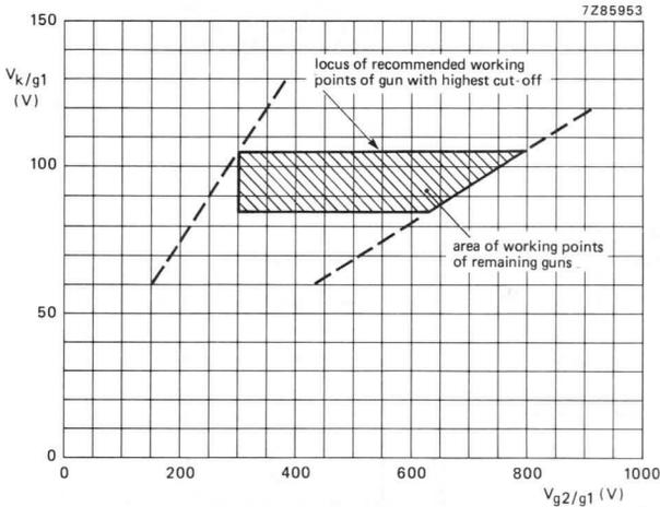
Fig. 12 Spot cut-off design chart.
