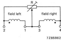
Fig. 2 Field coils.
