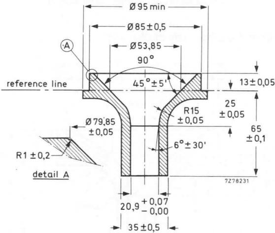
Fig. 2 Reference line gauge for 90° deflection angle.
