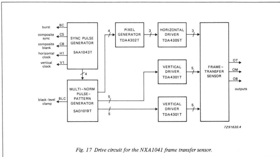
Fig. 17 Drive circuit for the NXA1041 frame transfer sensor.
