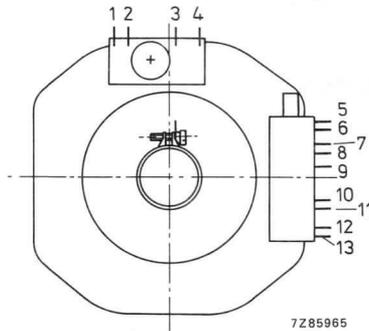
Fig. 3 Terminal location of deflection coils.
