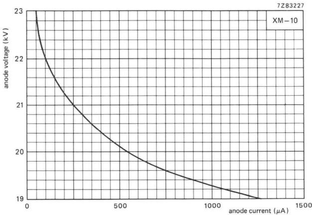
0,5 mR/h isoexposure-rate limit curve, according to JEDEC94, measured according to TEPAC103A.
