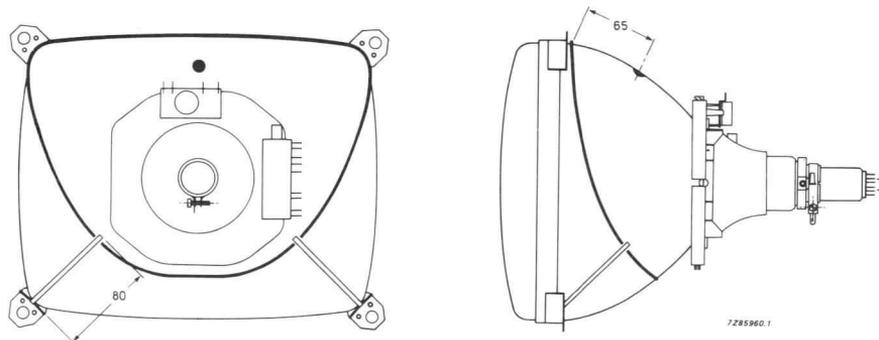
Fig. 21 Position of degaussing coil on the display tube; dimensions are given in mm.
