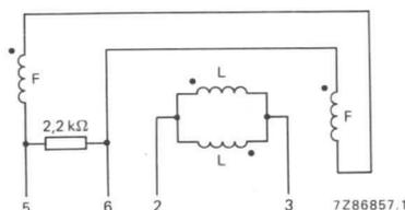
Fig. 2 Connection diagram, L = Line, F = Field.
