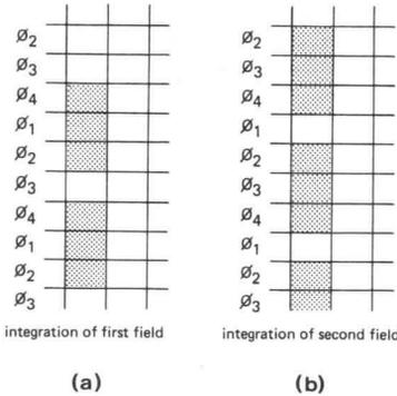
Fig. 3 Interlacing of the sensor.
