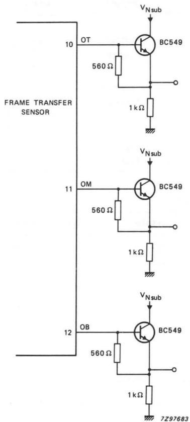
Fig. 5 Output buffer for measurements.
