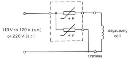
Fig. 19 Degaussing circuit using dual PTC thermistor.
