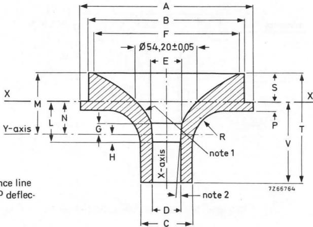
Fig. 1 Reference line gauge for 110° deflection angle.
