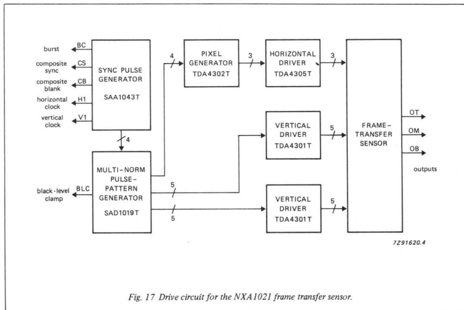
Fig. 17 Drive circuit for the NXA1021 frame transfer sensor.
