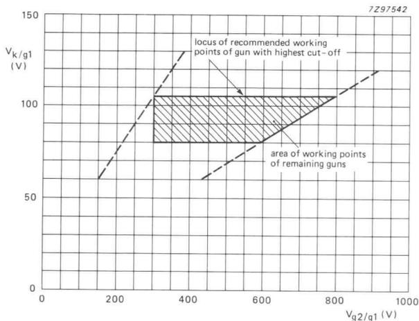
Fig. 13 Spot cut-off design chart.
