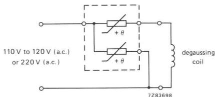
Fig. 22 Degaussing circuit using dual PTC thermistor.
