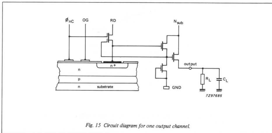
Fig. 15 Circuit diagram for one output channel.
