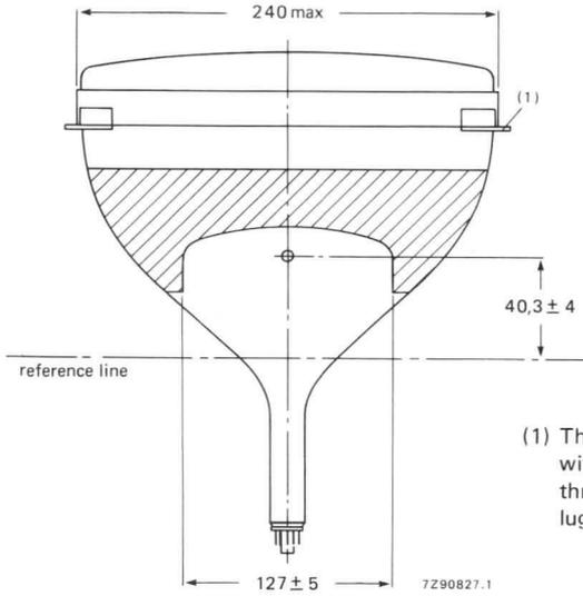
(1) The displacement of any lug with respect to the plane through the other three lugs is max. 1,5 mm.
