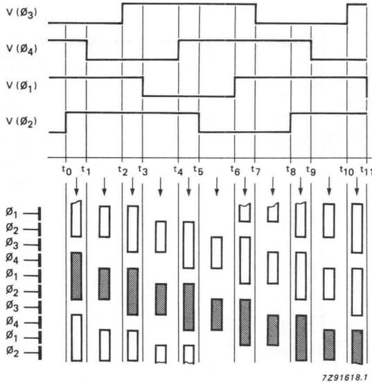
Fig. 2 Charge transport in the vertical direction.
