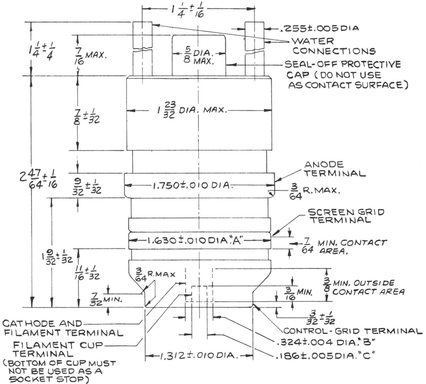
**CONCENTRICITIES:** The following total indicator readings are measured with respect to a centerline determined by the centers of the anode terminal and control grid terminal.
