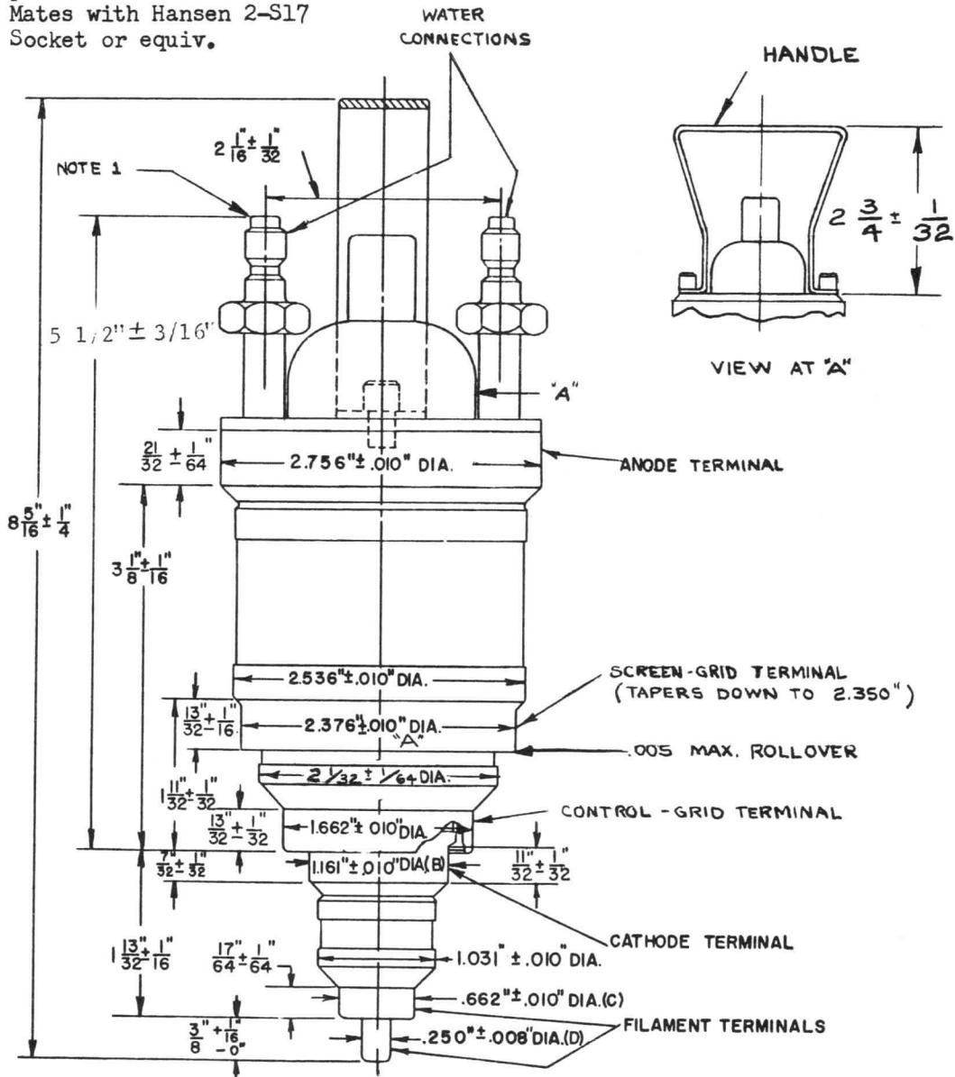
The following indicator readings are measured with respect to a centerline determined by the centers of the anode terminal and control grid terminal.
