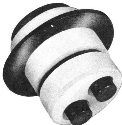
The 7077 is a high- $\mu$  triode of ceramic and metal planar construction primarily intended for use as an r-f amplifier in the UHF range. It features an extremely low noise figure throughout its frequency range. The 7077 is especially suited for use where unfavorable conditions of mechanical shock, mechanical vibration, and nuclear radiation are encountered.
