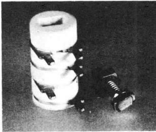
The 8083 is a high- $\mu$  triode of ceramic-and-metal planar construction primarily intended for radio-frequency amplifier service from low frequencies into the ultra-high frequency range.
