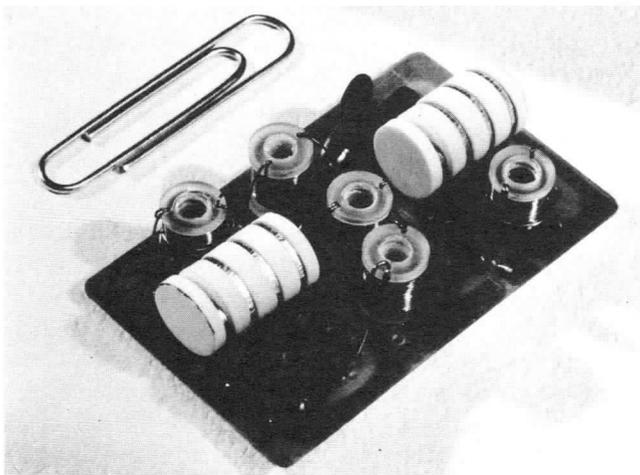
A complete cascode circuit showing two soldered-in titanium metal ceramic triodes. This circuit features small size and weight through the elimination of sockets and the use of printed circuit techniques.
