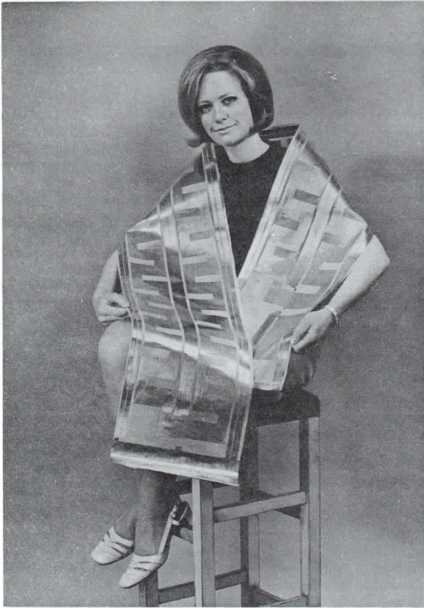
Not a new line in stoles, but illustrating the general appearance of a length of printed conductors before winding.
