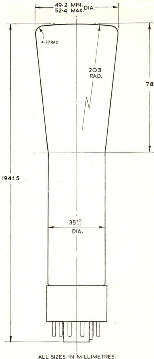
**Note 1.** When viewing the screen with the tube positioned such that Pin No. 1 is uppermost, a positive voltage applied to the terminal X1 will deflect the spot to the left and a positive voltage applied to the terminal Y1 will deflect the spot upwards.
