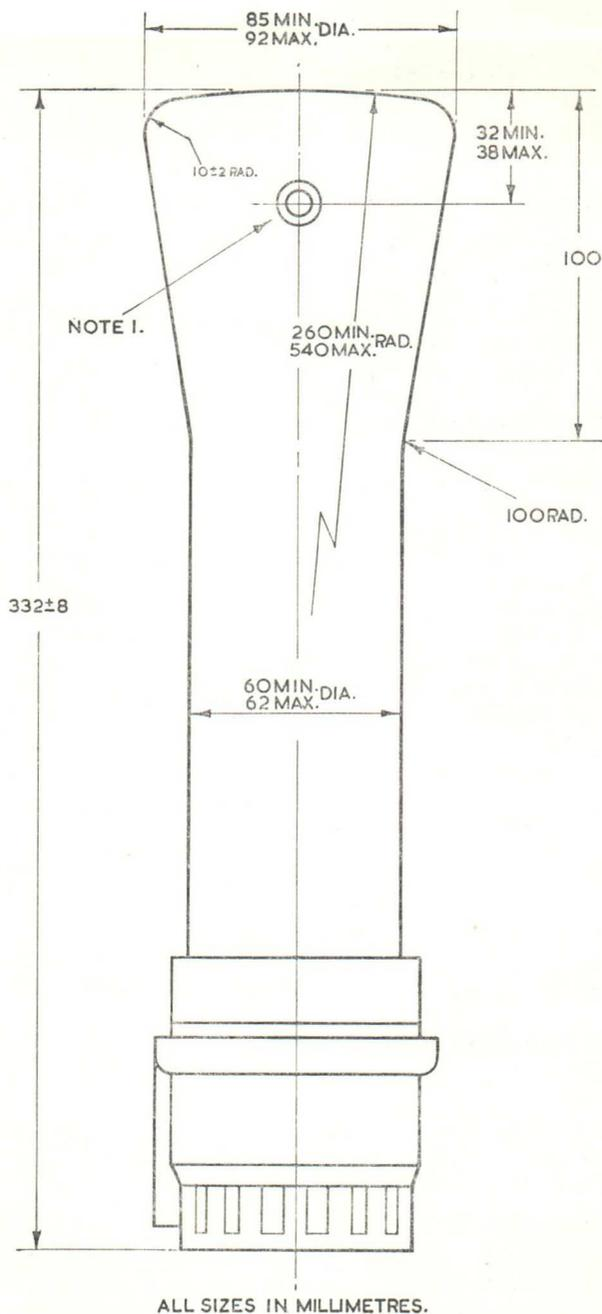
**Note 1.** When viewing the screen with the tube positioned such that the base spigot is uppermost, a positive voltage applied to the terminal X1 will deflect the spot to the left and a positive voltage applied to the terminal Y1 will deflect the spot upwards.
