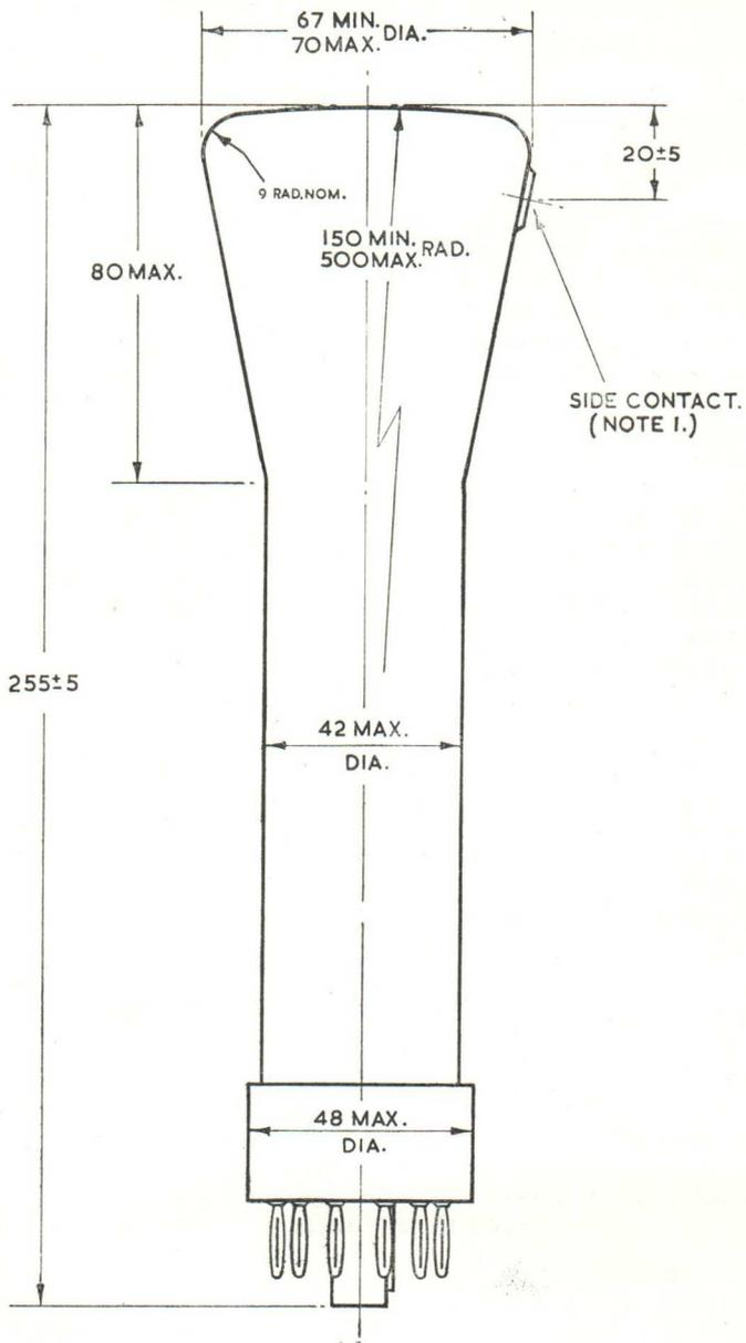
**Note 1.** When viewing the screen with the tube positioned such that the base spigot is uppermost, a positive voltage applied to the terminal X1 will deflect the spot to the left and a positive voltage applied to the terminal Y1 will deflect the spot upwards.
