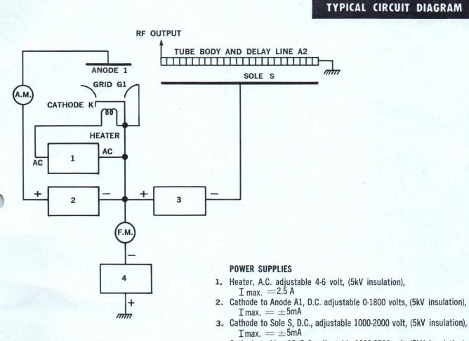
4. Cathode to Line A2, D.C. adjustable 1000-3500 volt, (5kV insulation),  $\rm Imax. = 250 \, \rm mA$
